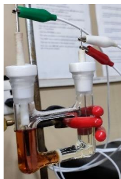
Figure: a) (C_6(PPh_3)_2-NDI) Crystals grown in Electro-crystallization setup in MeCN b) X-ray crystal structure of (C_6(PPh_3)_2-NDI) ORTEP representation c) UV-vis-NIR spectra of (C_6(PPh_3)_2-NDI) in DCM
